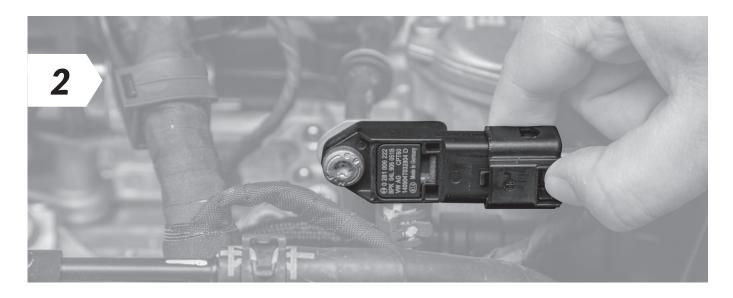
· Disconnect the turbo boost pressure sensor
