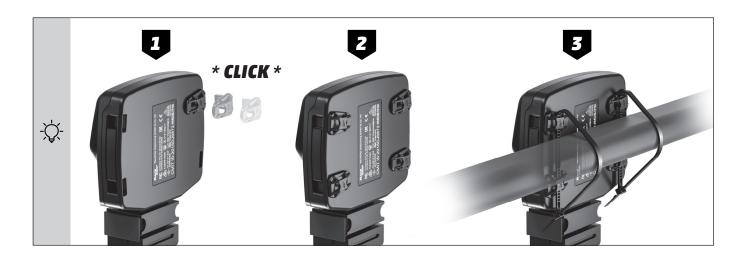
• If you need to remove the RaceChip at a later date, you can simply release the clips and do not have to cut any cable ties.
