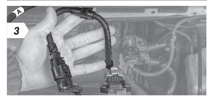
• Now connect the end of the RaceChip wiring harness marked "**A**" to the disconnected connector and the other end to the sensor.
